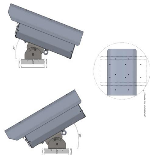
You will find a 1:1 template of placement of the holes for mounting on the last page of this document. You can print it and use it for drilling holes into the wall where the bracket will be mounted.
