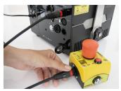
**B:** Connect the Emergency STOP Remote to the socket labelled as REMOTE INPUT with a supplied 3-pin XLR cable.
