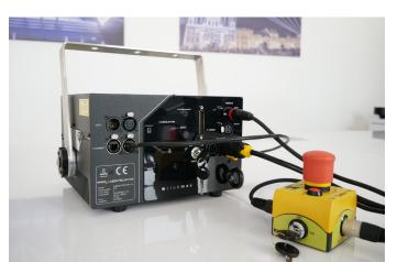
4. After the Emission Delay Period, the laser projector will be ready to start the emission.
