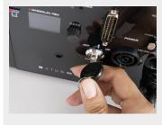
**A:** Turn laser system safety key to ON position.
