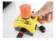
**B:** Press the START button on the E-STOP Remote.
