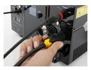
**D:** Use supplied Neutrik powerCON TRUE1 power cable to connect the laser system to mains power supply using the INPUT connector.
