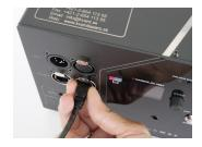
**A:** To control the system with an external signal such as Ethernet, DMX or ILDA, plug the corresponding cable into its designated connector at the back of the unit.
