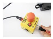
**C:** Insert the Remote Interlock Bypass dongle to the E-STOP Remote to disable the interlock (the USA only).
